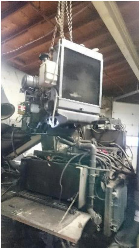
Pictured above, the old motor being removed from the street sweeper. That part was on a platform with many other parts attached, including the radiator (the large black part in the foreground). DPW personnel successfully detached and removed the old motor, attached the new motor and installed it back in the sweeper.
